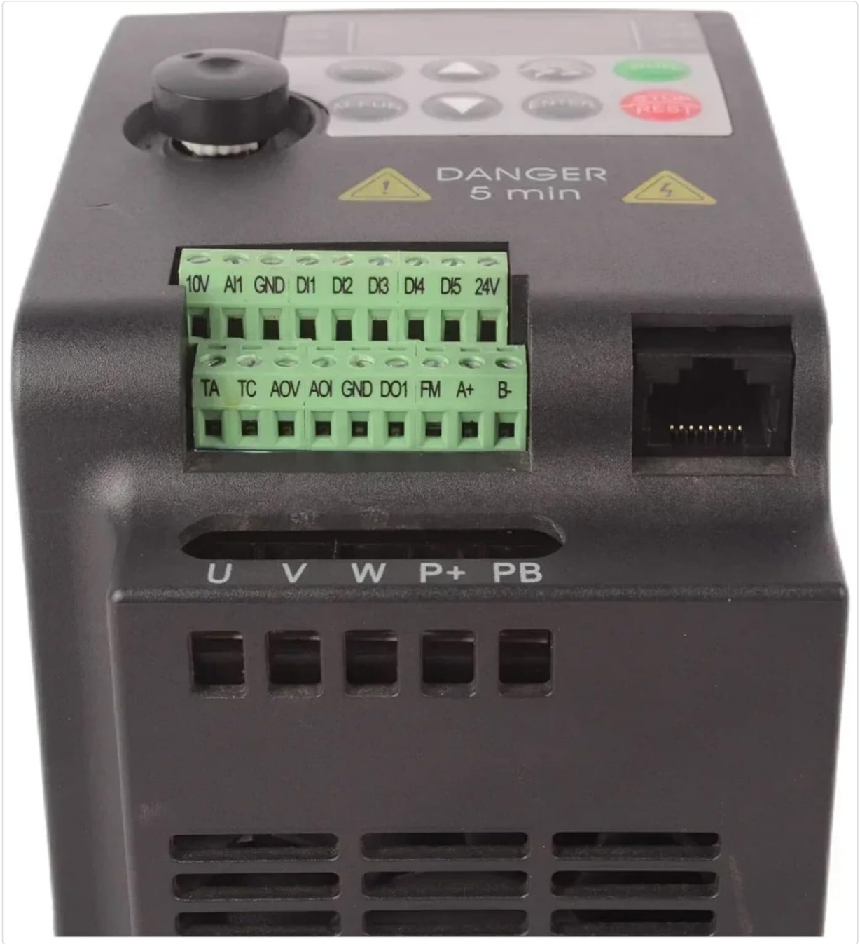
Figure 5.2: Detailed view of the VFD's control and power terminals.
