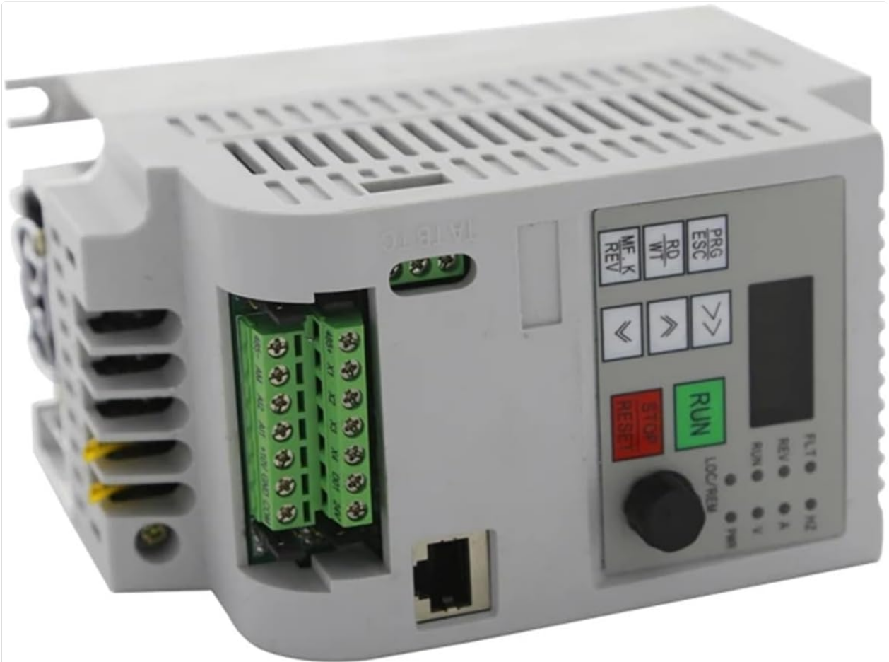
Figure 3.2: Angled Front View. An angled view of the VFD, highlighting the control panel and the accessible terminal blocks at the bottom for input/output connections. The ventilation grilles on the side are also visible.
