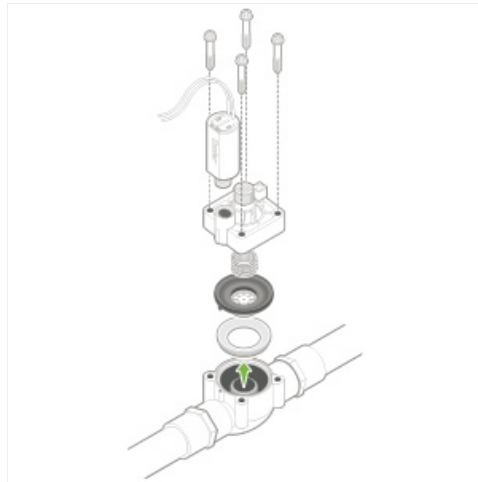
Image: Exploded view of valve components, showing the bonnet and body.
