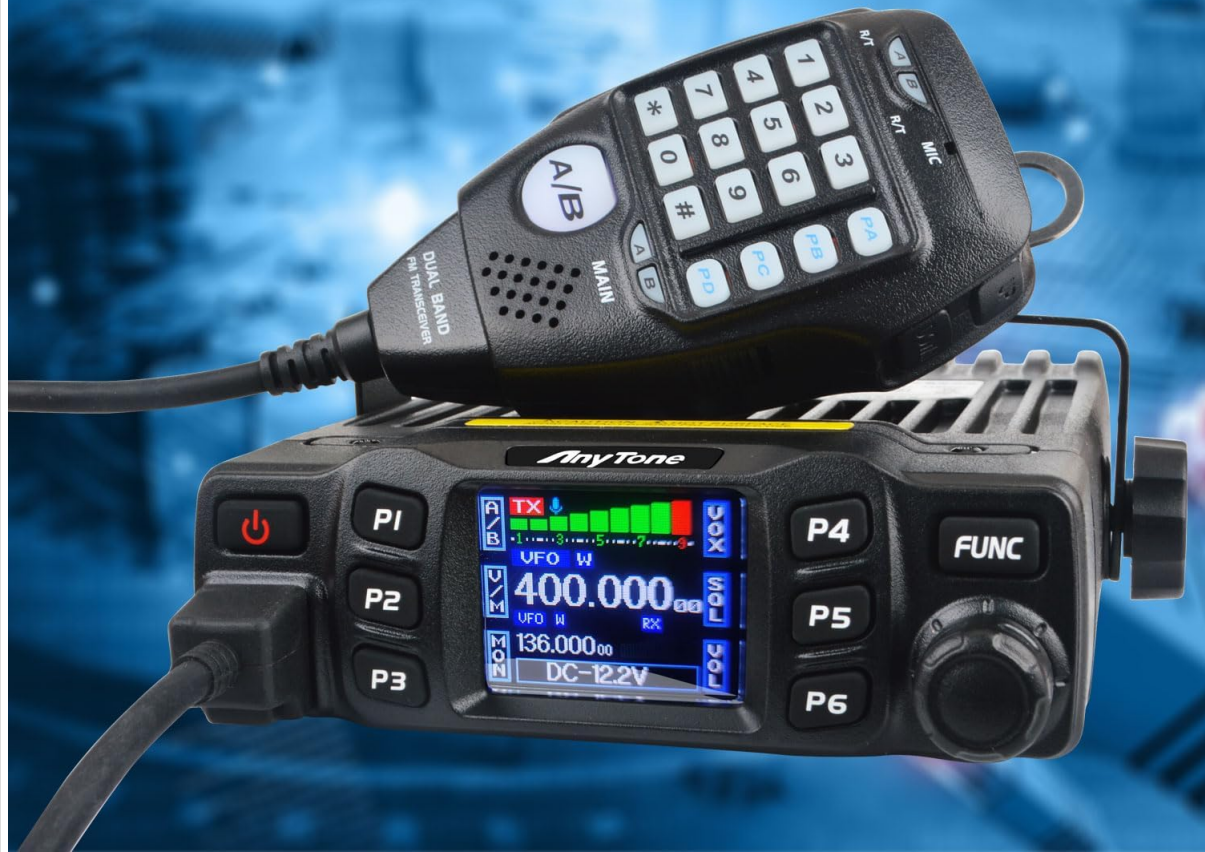
Figure 6: The radio display showing options for 200 programmable memory channels and settings for 52 groups of CTCSS tones and 1024 groups of DCS codes.
