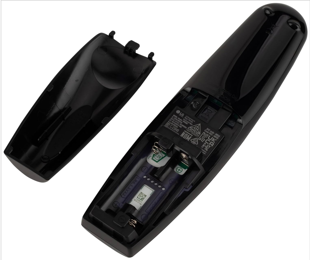
Image 2.1: View of the LG Magic Remote with the battery compartment open, illustrating correct AA battery placement.
