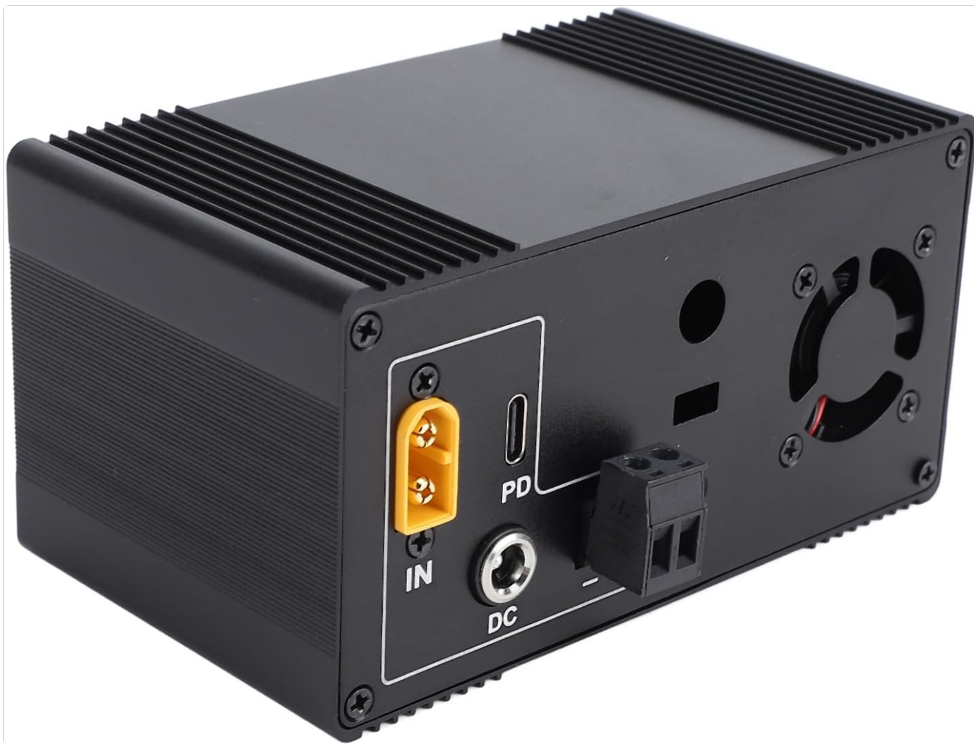
Figure 2: Rear input connections of the voltage regulator.
