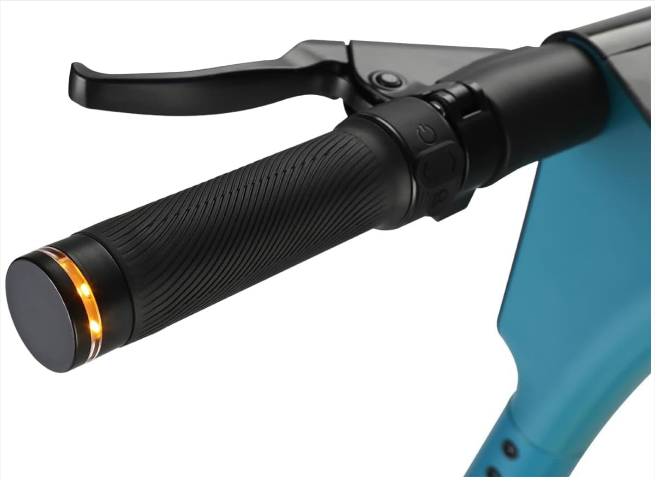
Image: Detailed view of the handlebar grip and brake lever, illustrating the control layout.
