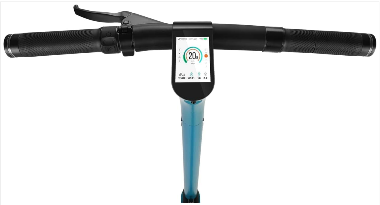
Image: Close-up view of the scooter's intelligent color display, showing speed, battery level, and other riding data.
