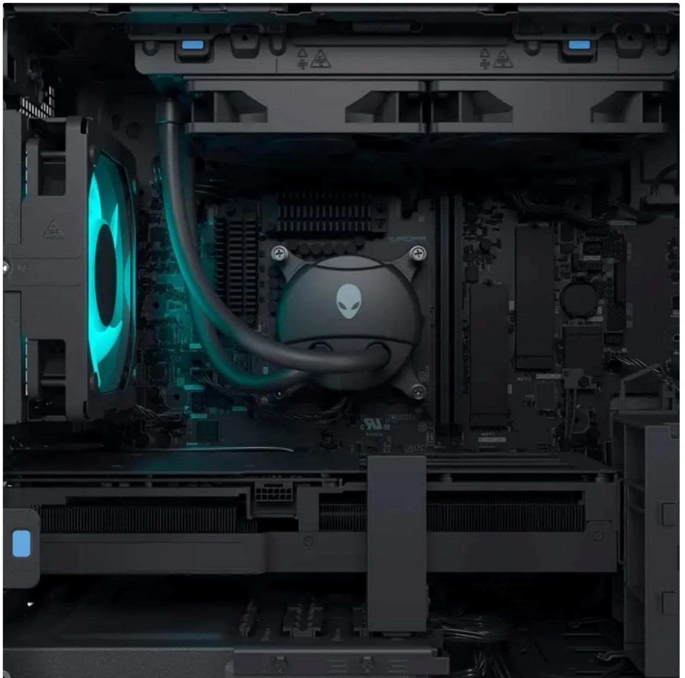
Figure 5.2: Internal view highlighting the liquid CPU cooling system and other components.
