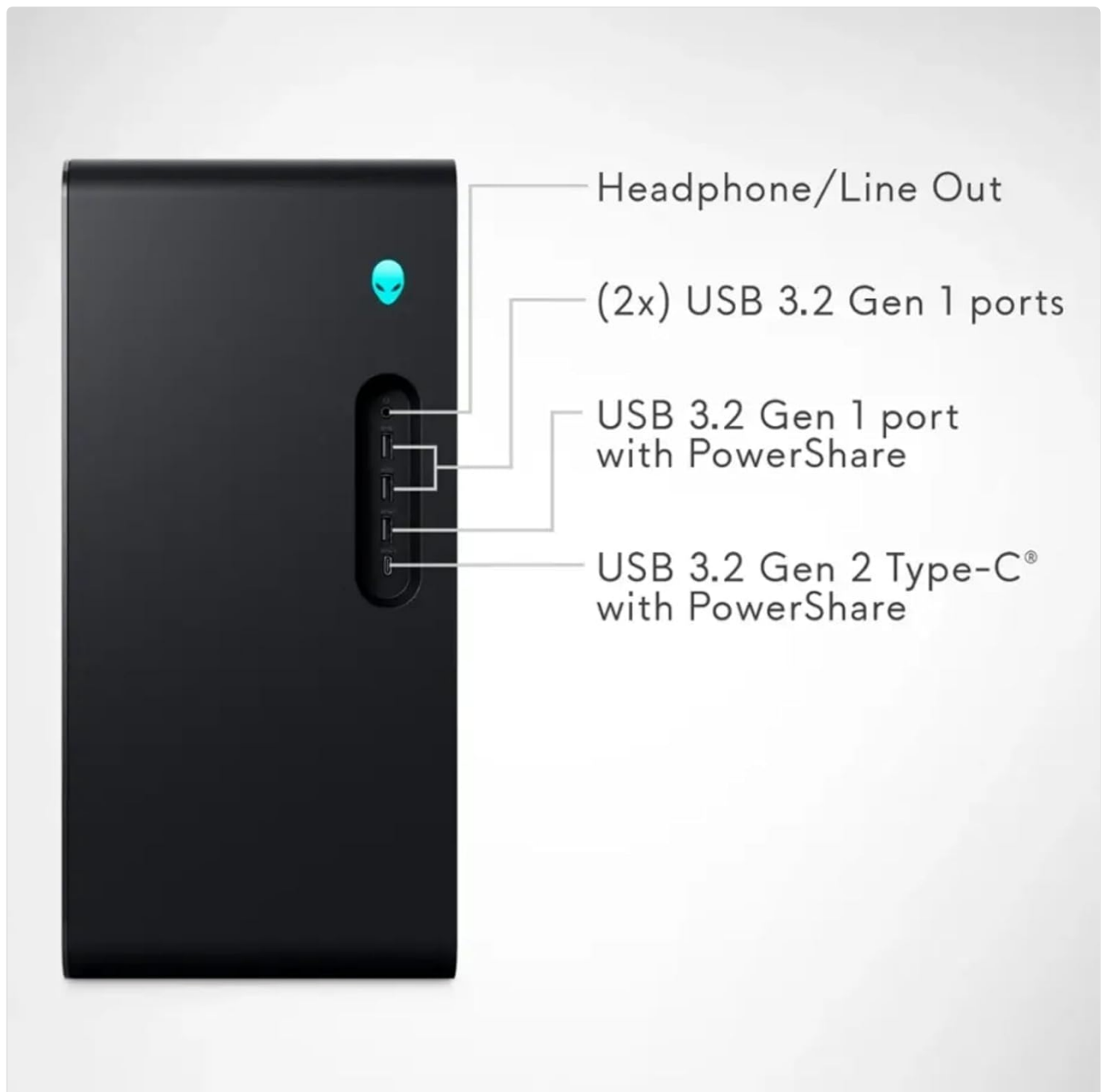
Figure 3.2: Front I/O ports including USB 3.2 Gen 1, USB 3.2 Gen 2 Type-C, and headphone/line out.
