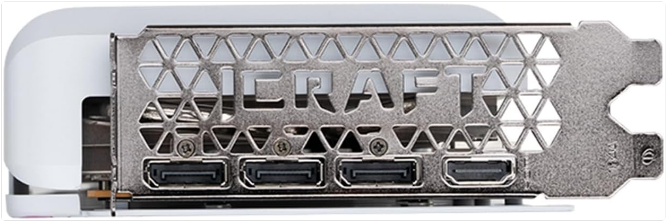
Image: Close-up of the graphics card's output panel, showing multiple DisplayPort and HDMI connections.
