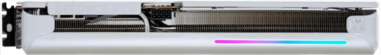
Image: Side view of the graphics card, revealing the heatsink fins and the integrated ARGB light strip.
