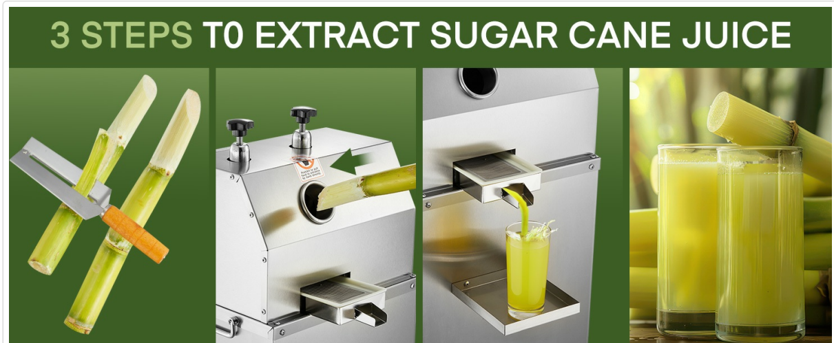
Figure 5: Visual guide illustrating the three main steps for sugarcane juice extraction: preparing the cane, feeding it into the machine, and collecting the fresh juice.
