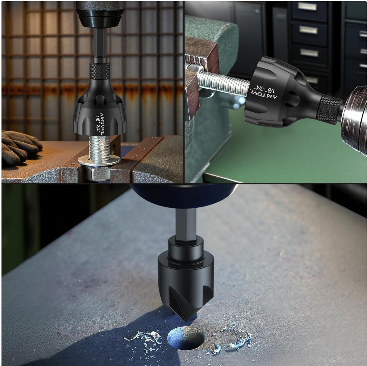
Figure 5.1: Images showing the external chamfer tool deburring a bolt and the countersink drill bit creating a chamfered hole in metal.
