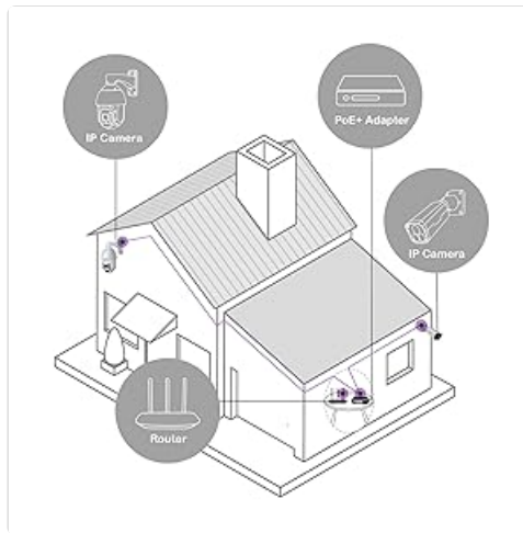
Figure 3.1: Typical Installation Diagram. This diagram illustrates how the camera can be integrated into a home network setup using a PoE+ adapter and router.
