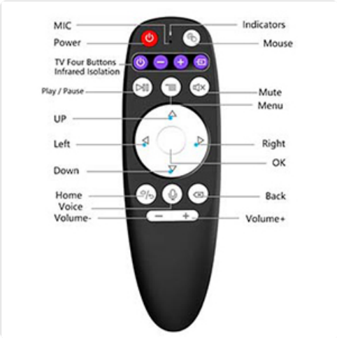
Image 4.1: A detailed diagram labeling each button on the BOXPOT G10S King remote control, including Power, MIC, Indicators, Mouse, TV Four Buttons Infrared Isolation, Play/Pause, Mute, Menu, Directional Pad (UP, Left, Down, Right, OK), Home, Voice, Volume-, Volume+, and Back.
