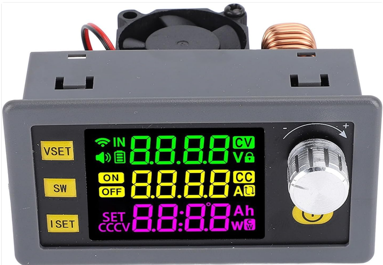
Figure 3.1: Front View of the Digital DC Regulator. This image shows the front panel of the SUNGOOYUE Digital DC Regulator, highlighting its vibrant multi-color digital display, control knob, and three function buttons (VSET, SW, ISET). The display shows input voltage (IN), output voltage (V), output current (A), power (W), and other status indicators.
