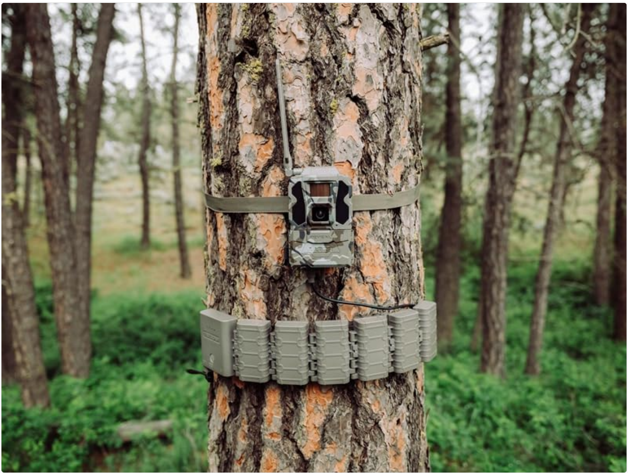
Figure 4: Camera mounted on a tree with an external battery pack.
