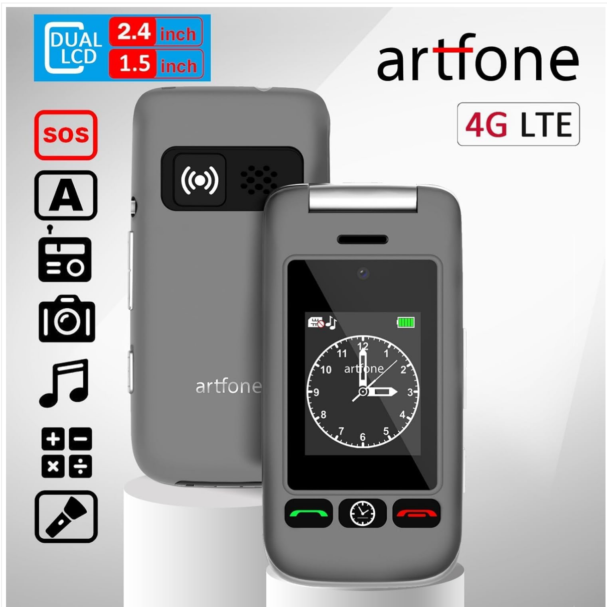
Image 1.1: The artfone G6 Pro 4G flip phone in its closed state, displaying both the front and back. Icons on the left highlight key features such as SOS, large buttons, camera, music, calculator, and flashlight.
