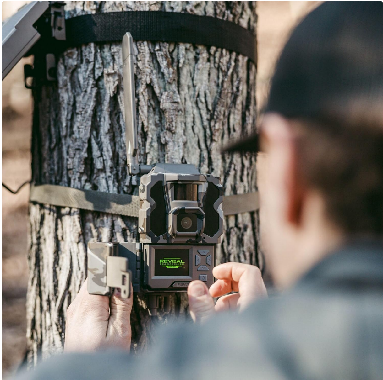
Image: Connecting the TACTACAM Battery Belt to the camera.
