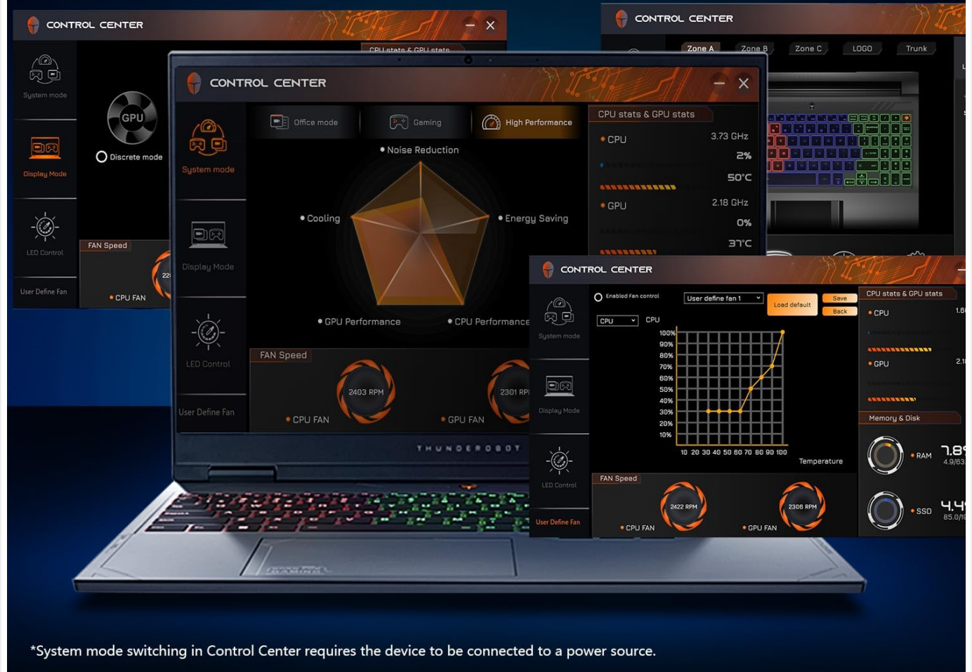
Figure 6: Screenshot of the Control Center software interface, showing options for performance modes and fan adjustment.
