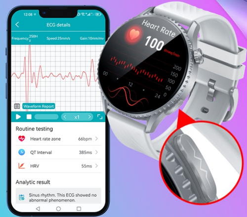
Figure 3.4: Real-time ECG monitoring interface on the smartwatch and the location of the electrode for measurement.
