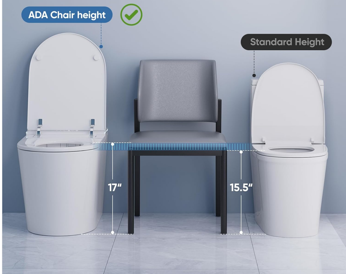
Figure 4.2.2: Comfortable Toilet Seat Height (ADA Compliant)
