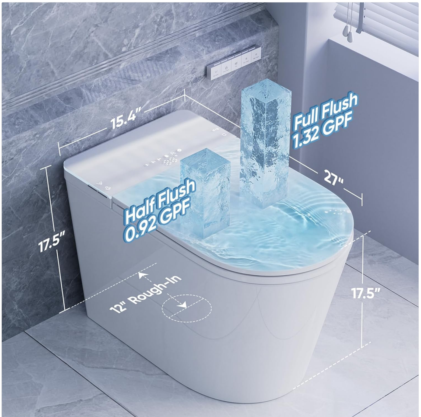
Figure 4.2.1: Product Dimensions and Flushing Volumes
