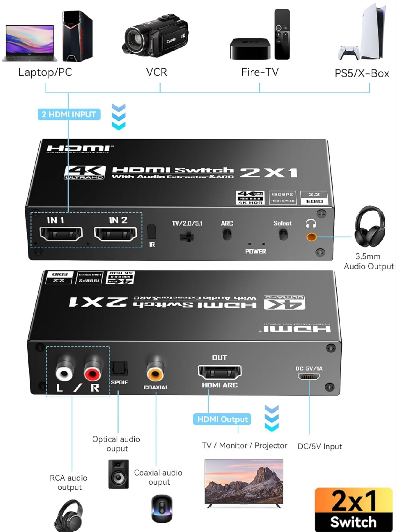
Image 4.1: Typical connection diagram.
