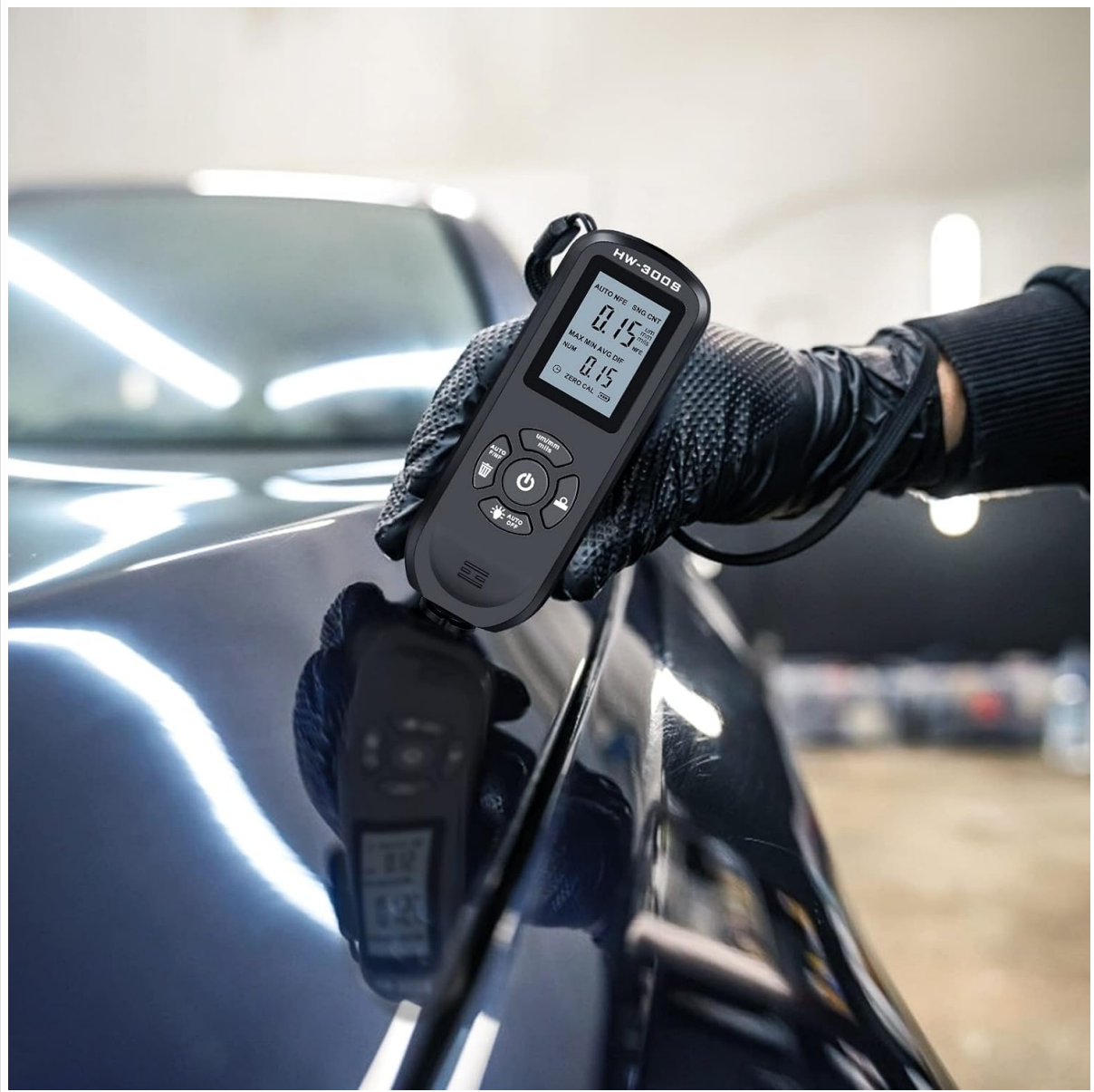
Figure 4: The HW-300S gauge in use, demonstrating how to measure coating thickness on a vehicle's painted surface.
