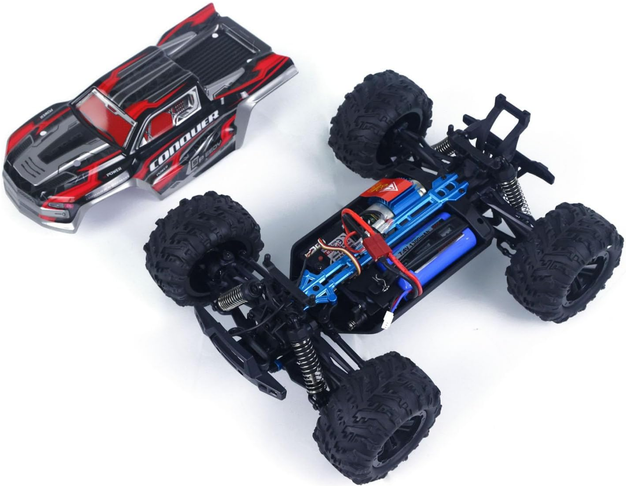
Image: Vehicle chassis with battery and motor visible, car shell removed.
