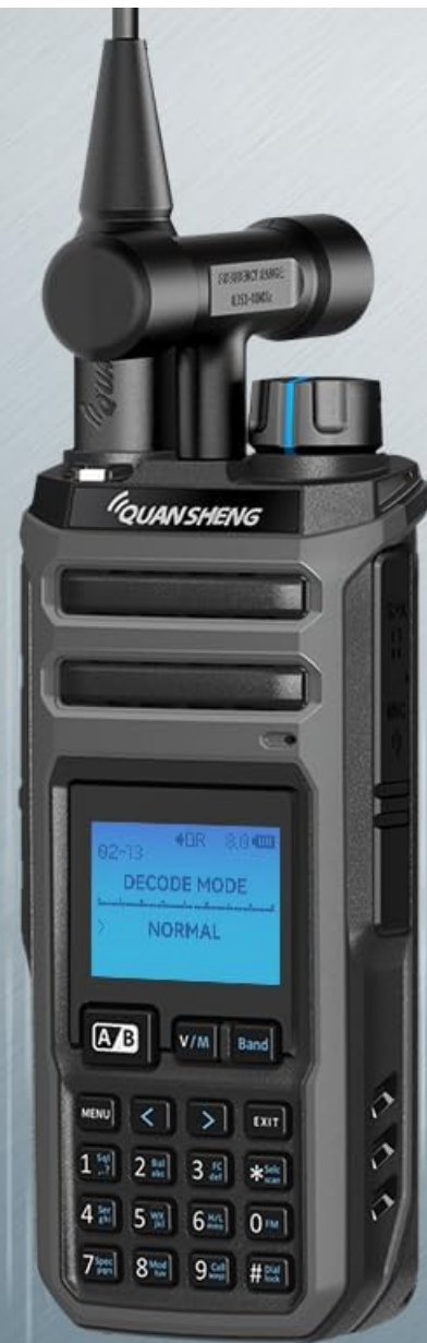
Figure 4.6: The walkie talkie supports three code breaking modes: Normal, Master, and Self-learning.
