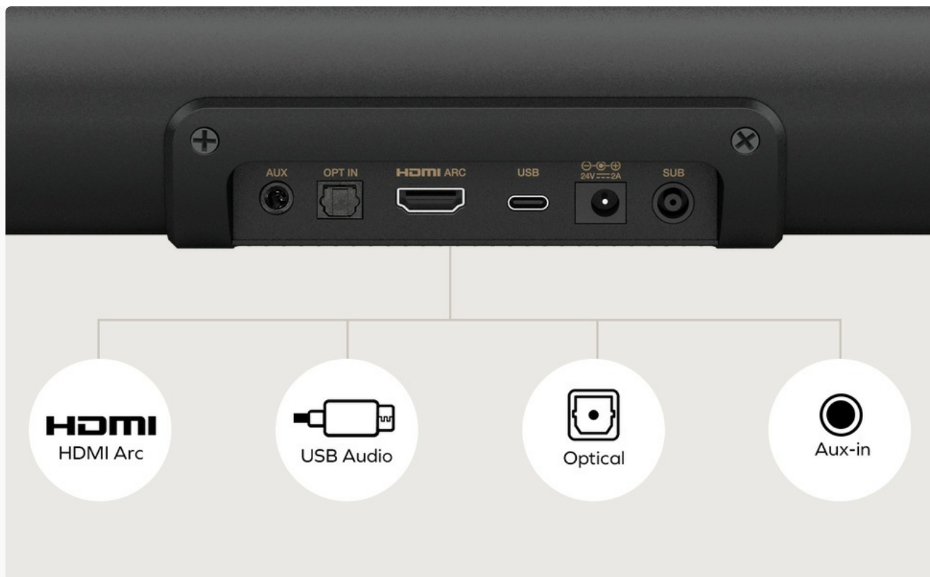
Image 2.3: A diagram illustrating the various connectivity options available on the Creative Stage Pro soundbar, including HDMI Arc, USB Audio, Optical, and Aux-in.
