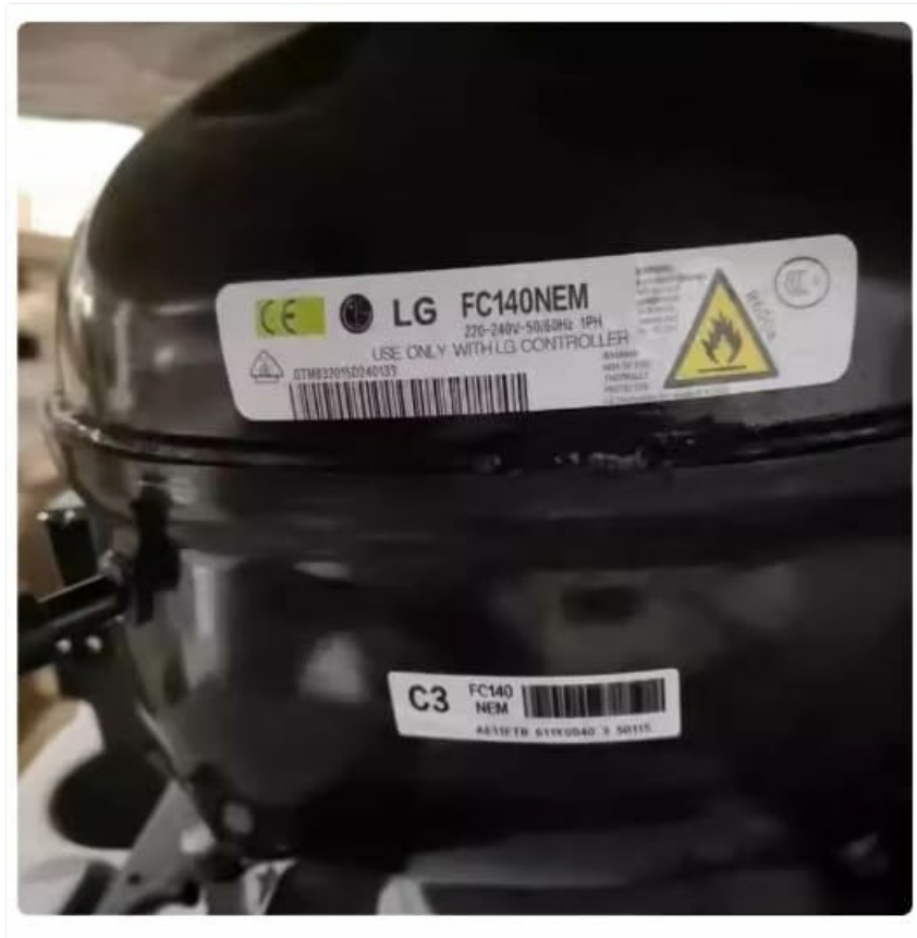
Image 1: Example of an LG compressor unit. Please note that while this image displays model FC140NEM, this manual specifically addresses the ZHRCLY replacement compressor for LG models including FC124NBME, FC150NAME, FC150NEM, and FLD165NBMA. The label indicates voltage (220-240V-50/60Hz 1PH) and a warning to "USE ONLY WITH LG CONTROLLER".
