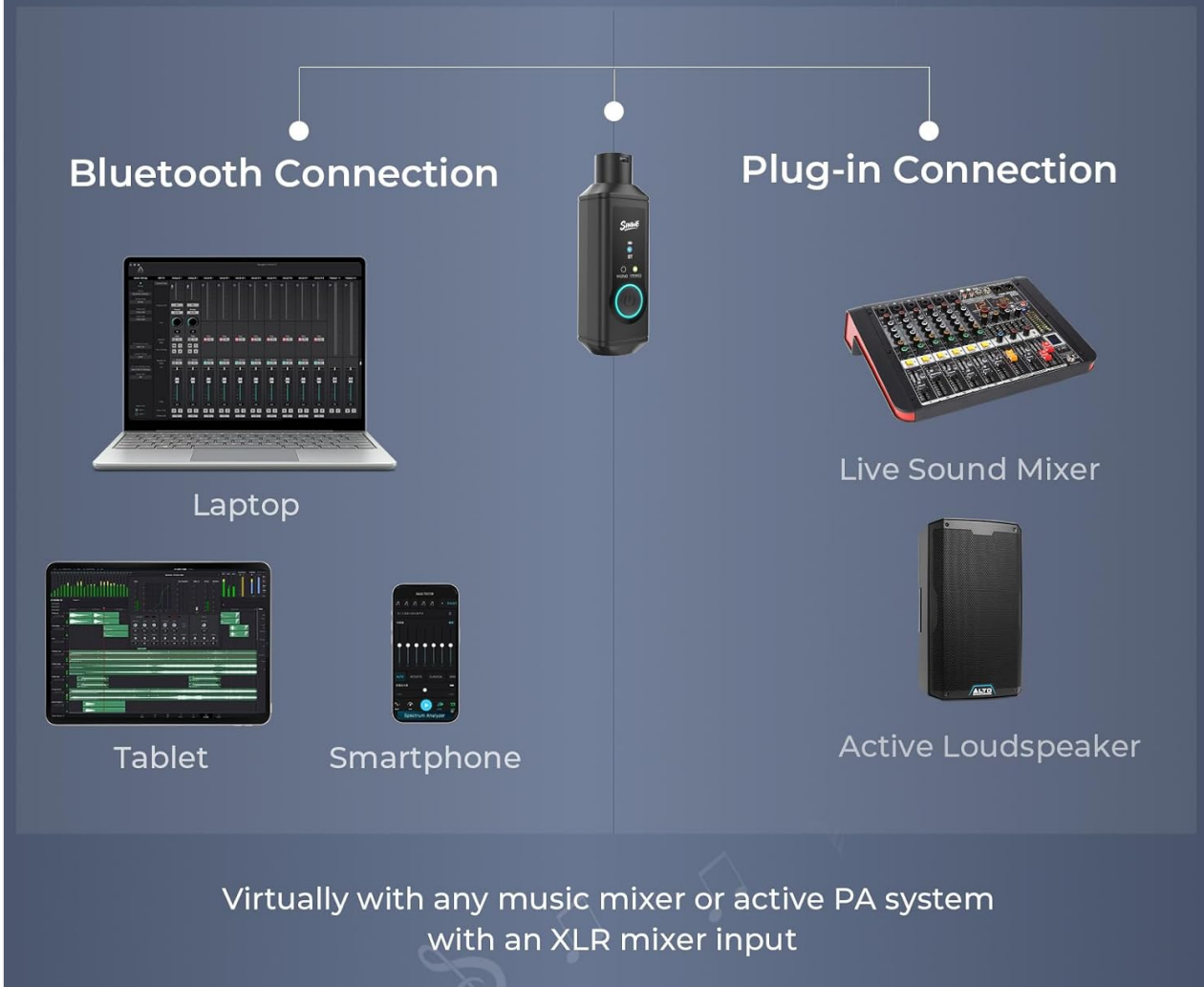
Figure 4: Diagram illustrating the various devices that can connect to the SINWE P16, including laptops, tablets, and smartphones via Bluetooth, and its connection to live sound mixers and active loudspeakers via XLR.
