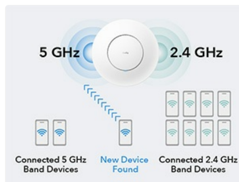
Image: A diagram showing how band steering directs devices to either the 5 GHz or 2.4 GHz band based on network conditions.
