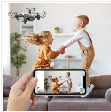
Image: A TEEROK T13 drone flying above a group of children, illustrating the concept of Headless Mode where the drone's orientation is relative to the controller.
