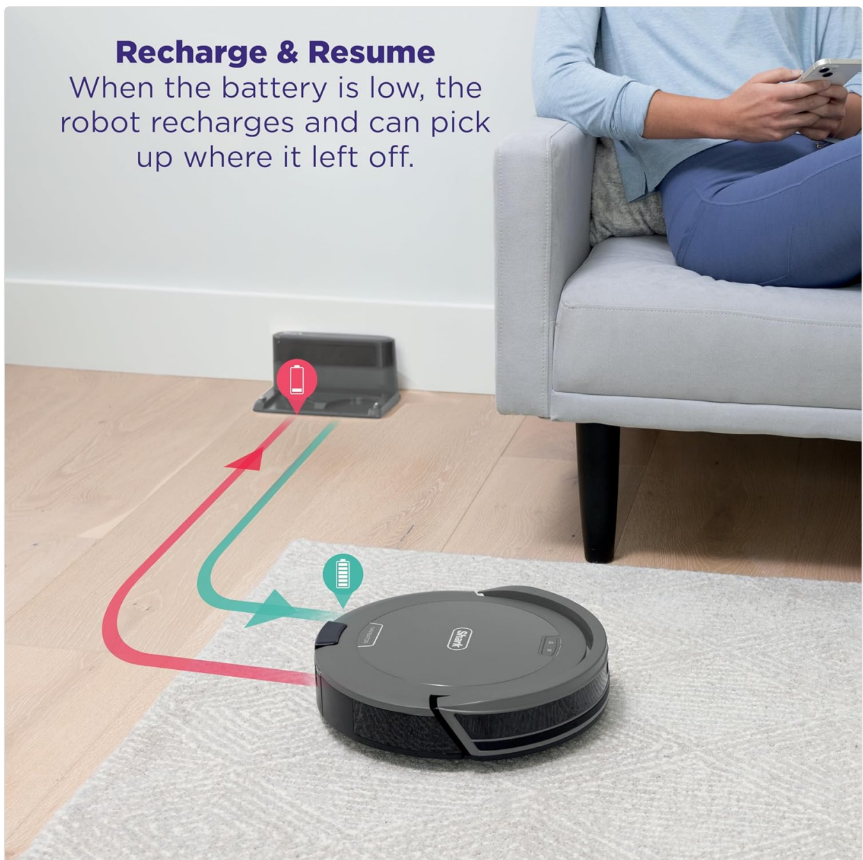
Image: The robot vacuum automatically navigating back to its charging station, illustrating the 'Recharge & Resume' feature. This ensures continuous cleaning without manual intervention.
