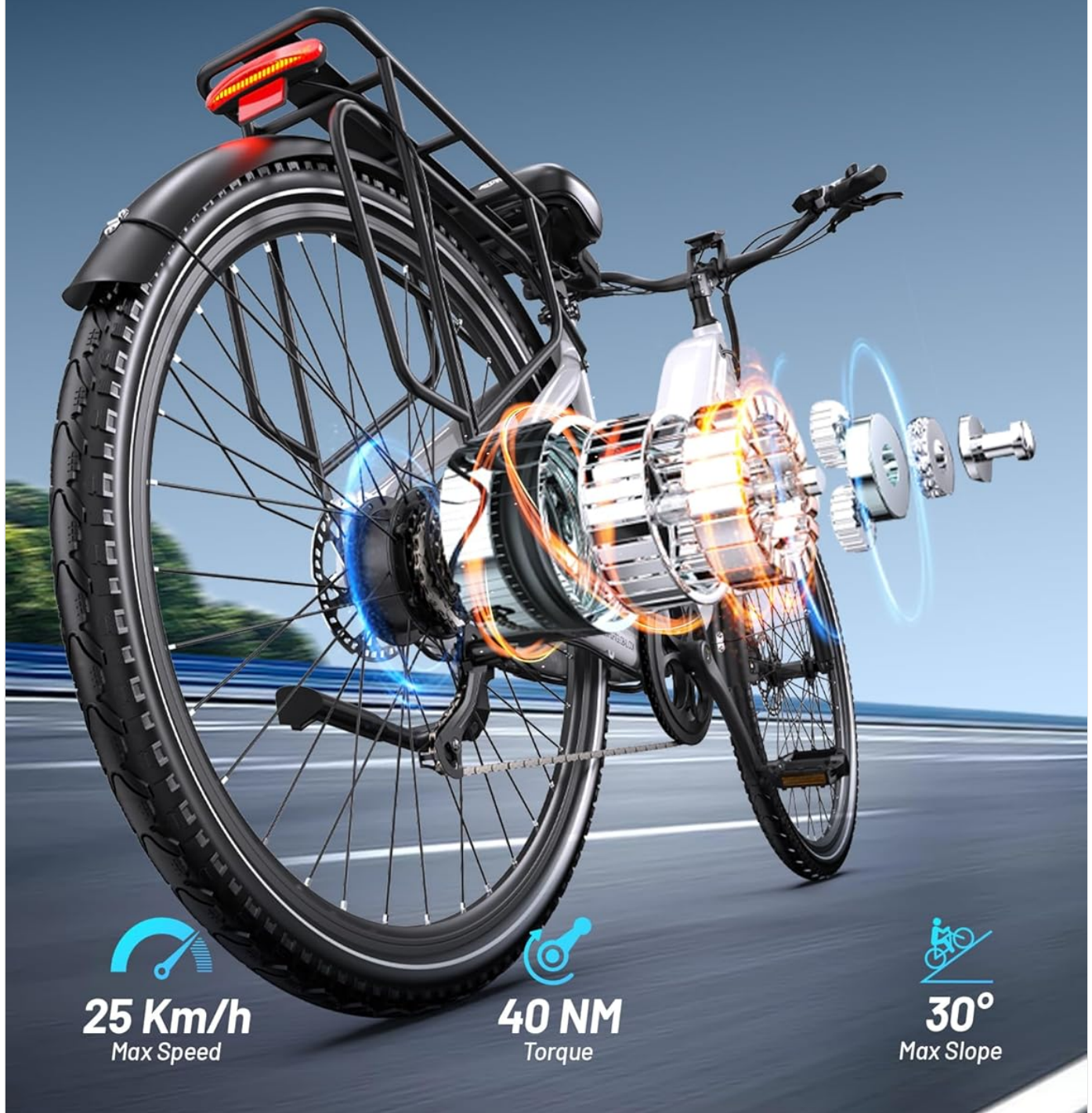
Figure 3.2: Detailed view of the 250W brushless motor and its integration with the rear wheel, showing maximum speed, torque, and climb angle capabilities.
