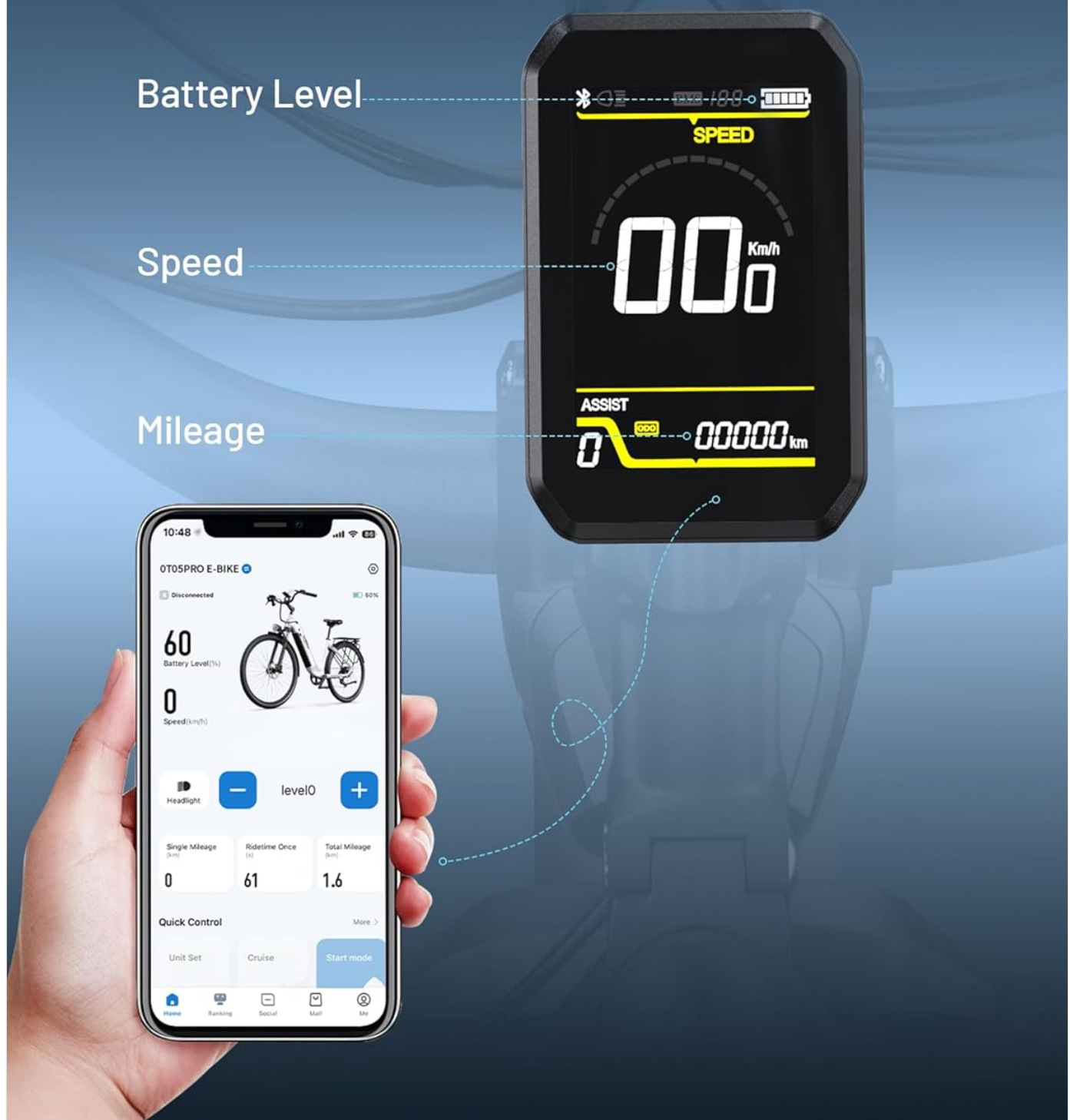
Figure 3.5: The bicycle's HD display showing key metrics and a smartphone screen demonstrating the companion app's interface for monitoring and control.
