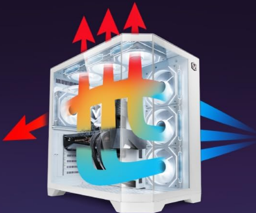
Image: An illustration of the inverse airflow design within the Vibox IV-570 PC case, showing how cool air enters and hot air is
