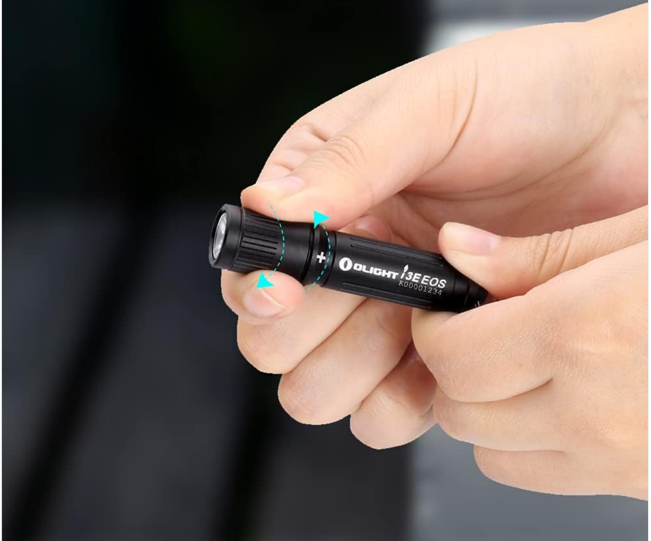
Image 3.2: i3E EOS demonstrating its easy switching mechanism by twisting the head.
