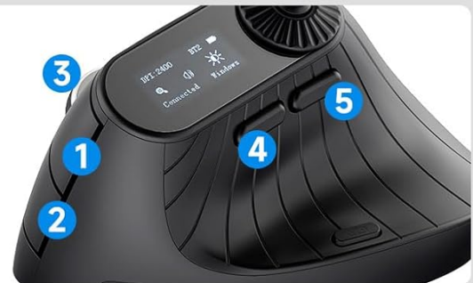
Image 3.3: The location of the 5 programmable buttons and an example of the customization software interface.
