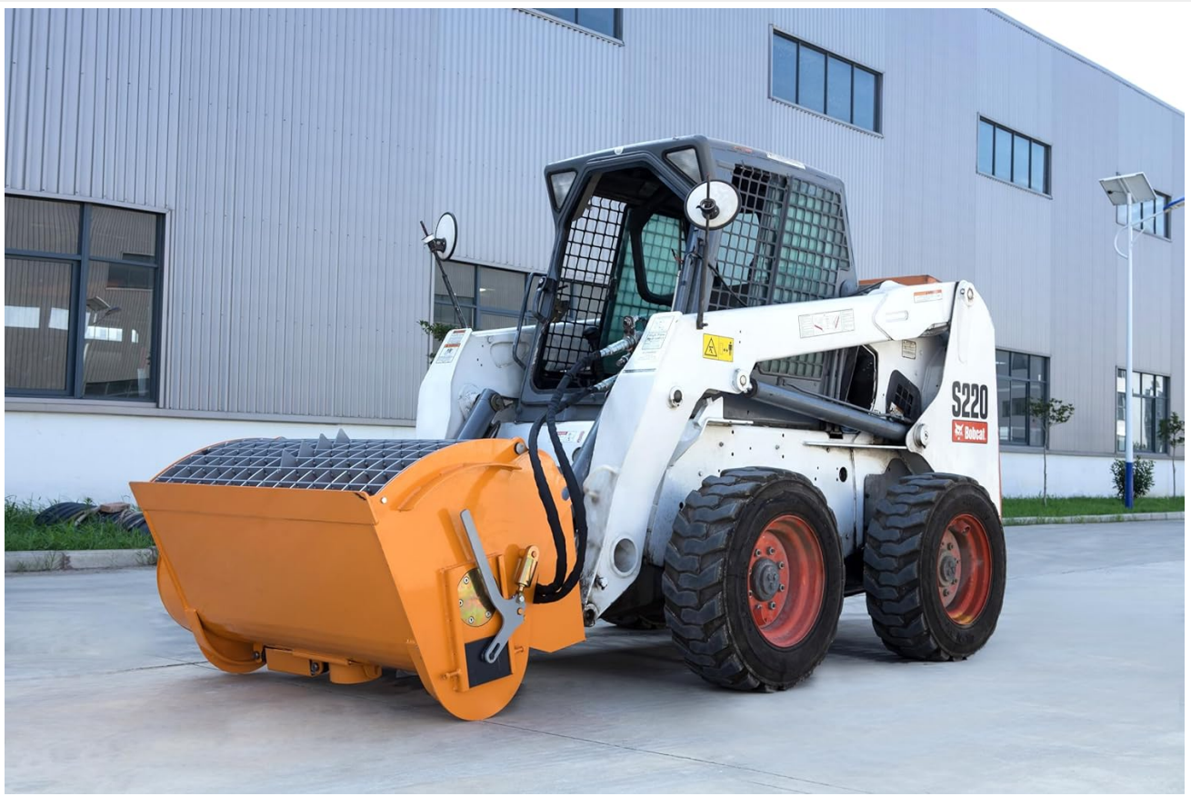
Figure 4.1: The LandHonor concrete mixer shown securely attached to a Bobcat S220 skid steer loader, demonstrating its operational configuration.
