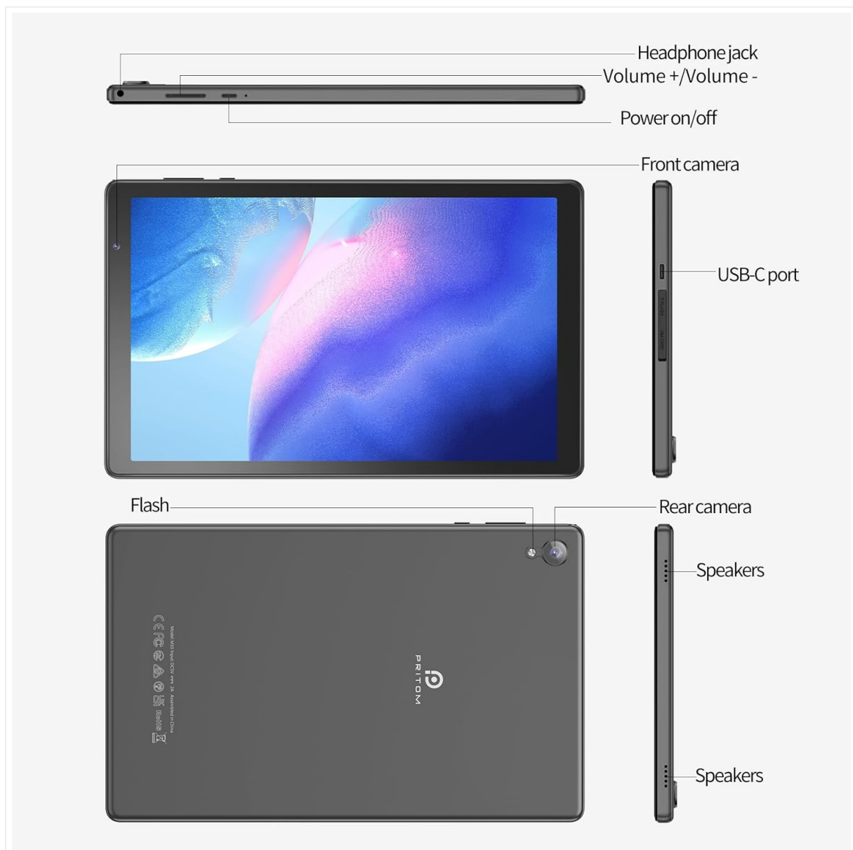
Image: Diagram illustrating the location of the headphone jack, volume buttons, power button, front camera, USB-C port, rear camera, flash, and speakers on the PRITOM TAB10 Tablet.
