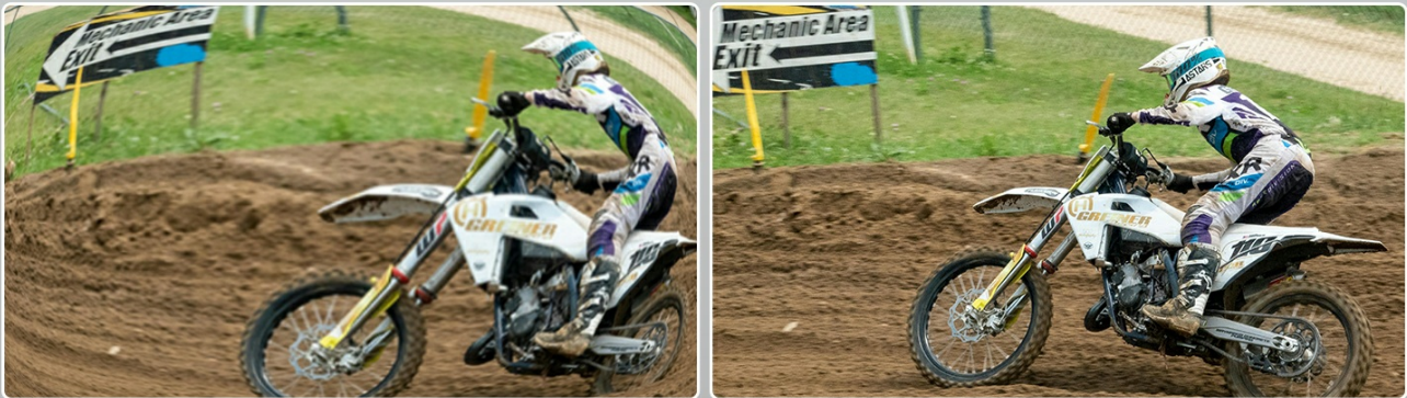
Image: A comparison showing the effect of LDC (Lens Distortion Correction) on the Apexcam X80pro. The left image shows a motocross rider with noticeable fisheye distortion, while the right image shows the corrected, flatter perspective.
