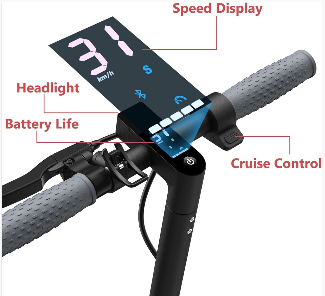
Figure 5.2: Handlebar display showing speed, battery life, headlight status, and cruise control.
