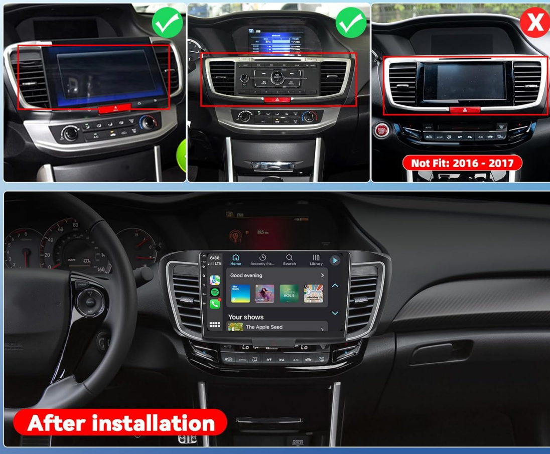
Figure 4.1: Dashboard compatibility for Honda Accord 9th Gen (2013-2017) 2.0L low-end version. Note: Not suitable for models with existing OEM Navi Screen.
