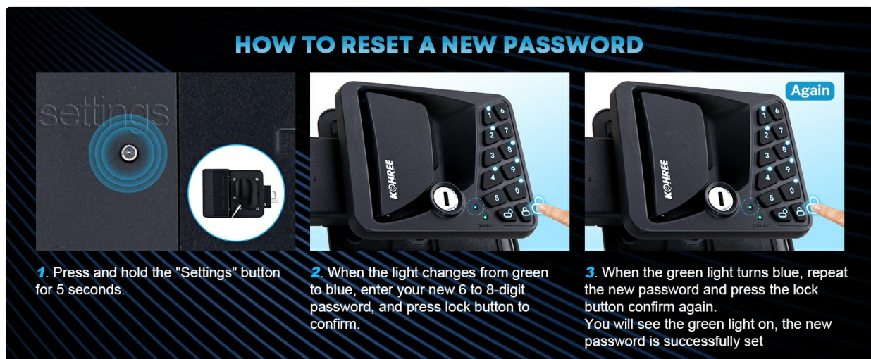
Figure 6: Step-by-step guide to resetting your keypad password.
