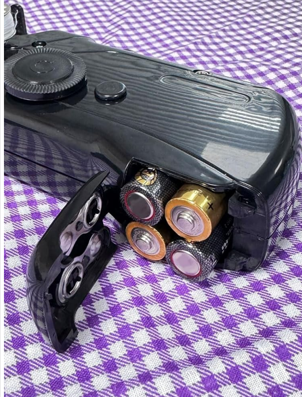
Image: The bottom of the sewing machine showing the battery compartment and the USB power input port.
