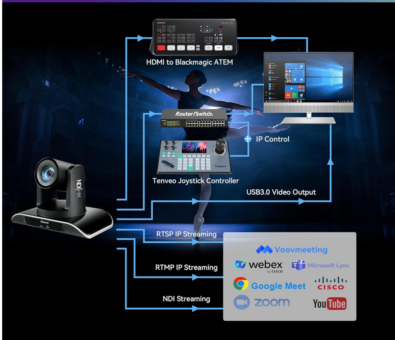
Image 5: A diagram illustrating the various connection options for the Tenveo NDI AI-Tracking PTZ Camera, including HDMI to Blackmagic ATEM, Router/Switch for IP Control, Tenveo Joystick Controller, USB3.0 Video Output, RTSP IP Streaming, RTMP IP Streaming, and NDI Streaming to platforms like Voovmeeting, Webex, Microsoft Lync, Google Meet, Cisco, Zoom, and YouTube.
