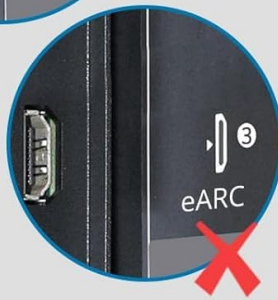
Image: A visual guide indicating the correct HDMI ARC port on a TV for connection, and explicitly marking standard HDMI and eARC ports as incompatible with this audio extractor.
