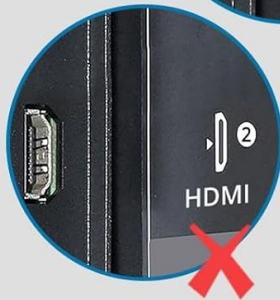
Image: A visual guide indicating the correct HDMI ARC port on a TV for connection, and explicitly marking standard HDMI and eARC ports as incompatible with this audio extractor.
