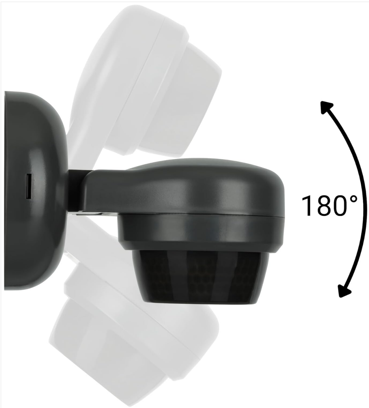
Image 4.2: The sensor head can be swiveled vertically by 180 degrees to adjust the detection area.
