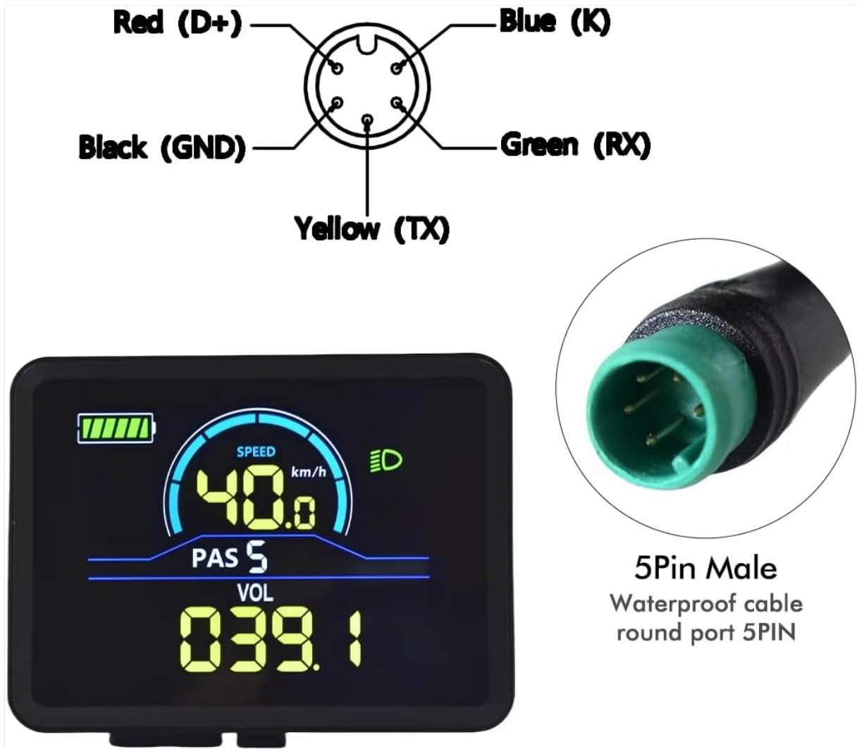
Image: A detailed diagram of the 5-pin male waterproof connector, showing the pin assignments (Red: D+, Blue: K, Black: GND, Green: RX, Yellow: TX), alongside the YL61F display.
