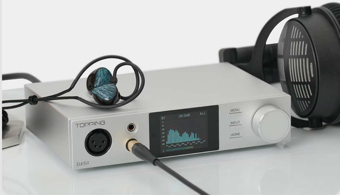
Image: The TOPPING DX5II unit with various headphones connected to its 6.35mm single-ended, 4.4mm balanced, and 4-pin XLR headphone output jacks, illustrating its broad compatibility.
