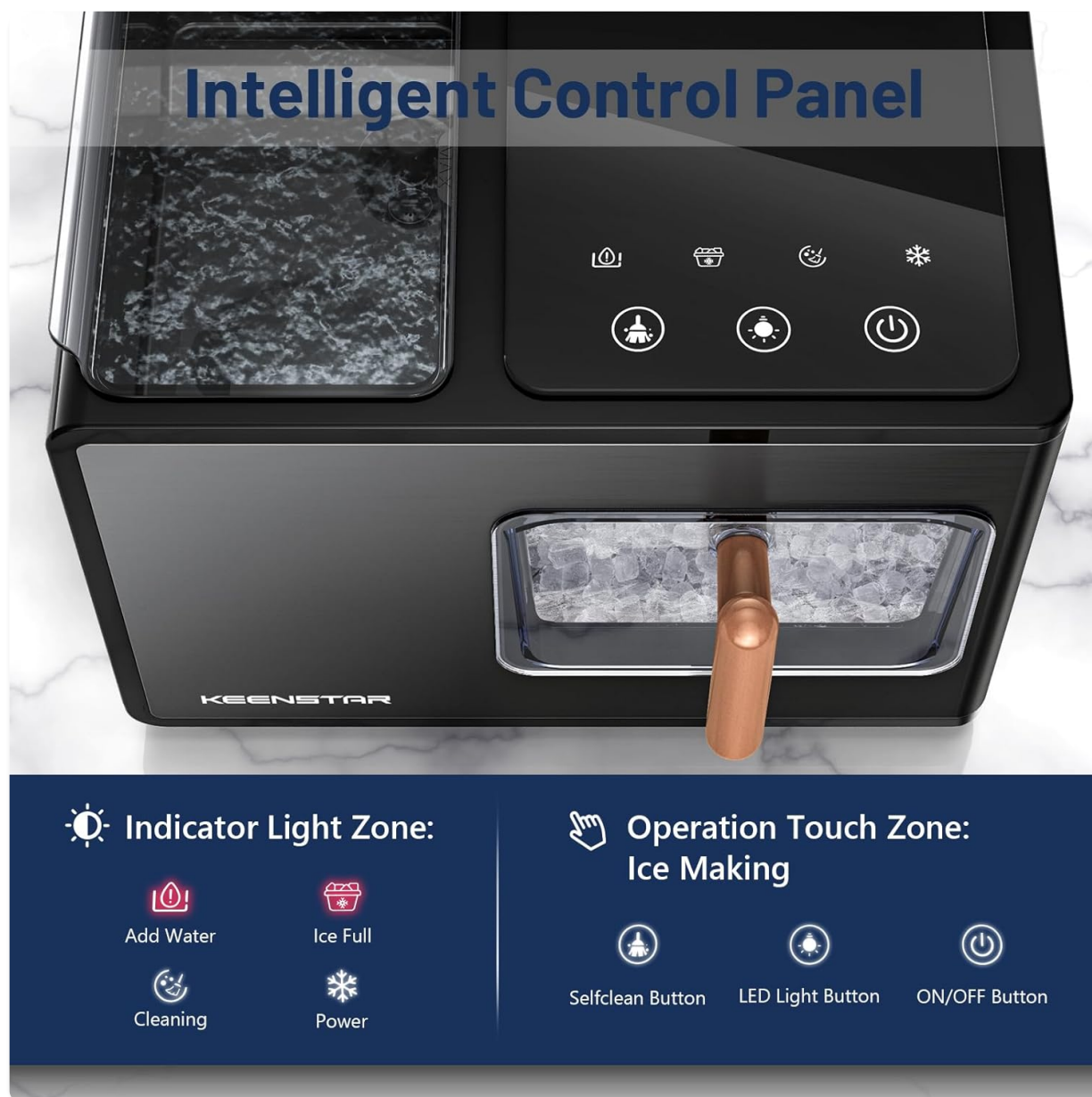
Image 3.1: A close-up view of the KEENSTAR ICN1580's intelligent control panel. It features indicator lights for 'Add Water', 'Ice Full', 'Cleaning', and 'Power', alongside touch buttons for 'Selfclean', 'LED Light', and 'ON/OFF'.
