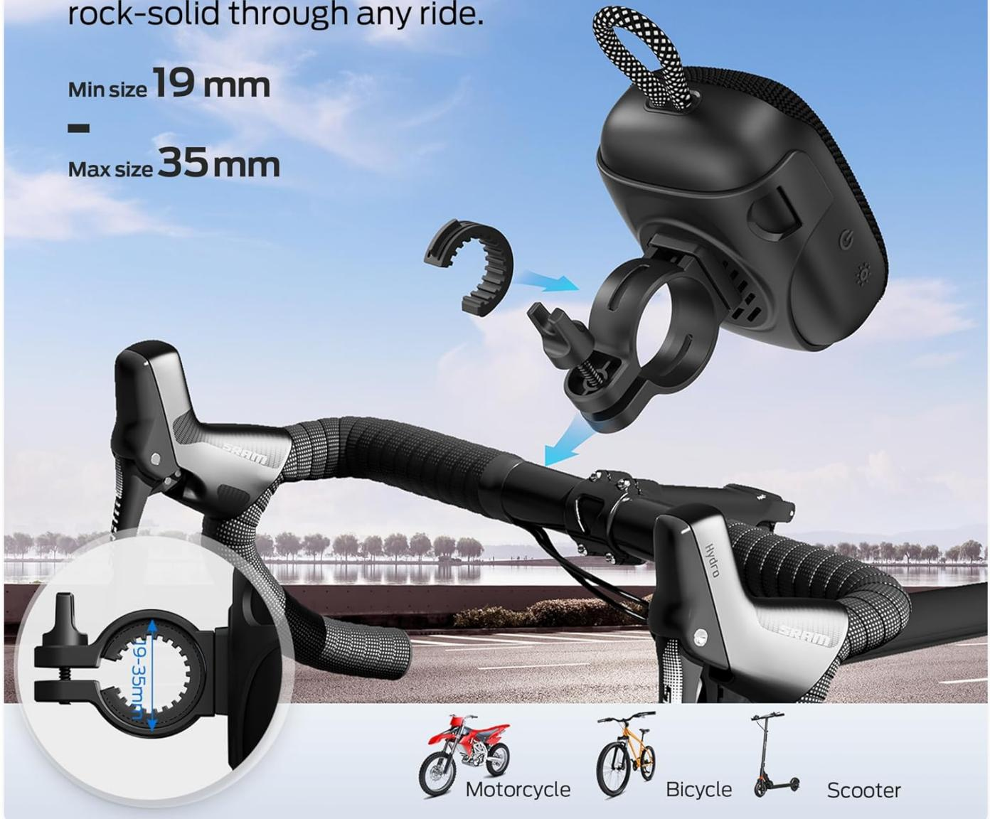
The Monster S300 comes with a secure handlebar mount. Slide the speaker onto the mount until it clicks into place. Use the provided rubber strips to ensure a snug fit on handlebars ranging from 19mm to 35mm in diameter. This mount is suitable for bicycles, motorcycles, and scooters.
