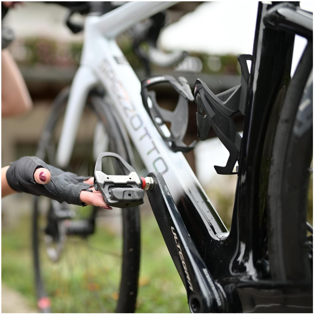
Image: Demonstrating the installation of the Assioma PRO RS-2 pedal onto a bicycle crank arm.
