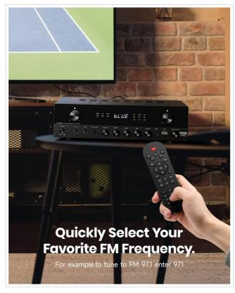
To tune into FM radio, select the FM mode. You can use the CH+ / CH- buttons to scan through stations or directly enter your desired frequency using the number pad on the remote control (e.g., for FM 97.1, enter 971).
