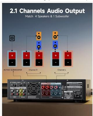
This diagram illustrates the connection of speakers and an active subwoofer to the Donner MAMP2 amplifier. Connect your main left and right speakers to the "Channel L" and "Channel R" terminals respectively. An active subwoofer can be connected to the dedicated "ACTIVE SUBWOOFER" output for enhanced bass.
